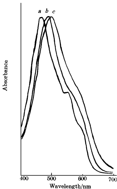
Fig.1 Absorption spectrum of HB, 5-Br-HB and 5,8-diBr-HB (a) HB (b) 5-Br-HB (c) 5,8-diBr-HB DMF as solvent
